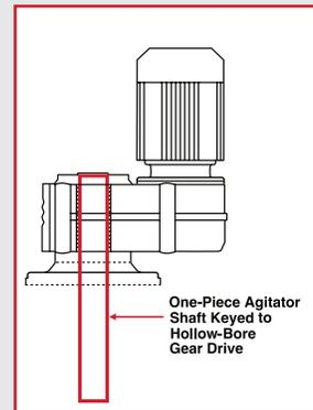
On Lee agitator drives, both the motor and the agitator shaft are keyed directly to the hollow-bore gearbox. This high-tolerance fit assures a secure linkup of the motor and agitator to the gearbox, eliminating potential for wear at these critical locations.
