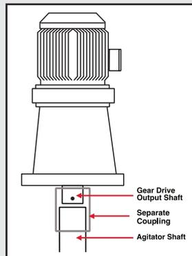
Most conventional drive units use a separate coupler to join the agitator shaft to the gear drive or motor shaft. Over time, this coupler can eventually loosen, requiring service and production downtime.
